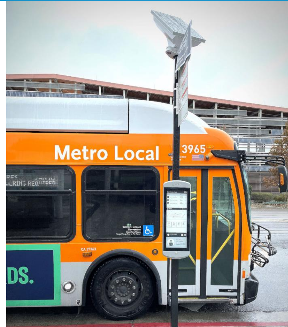
Metro bus stop with e-paper screen & solar
